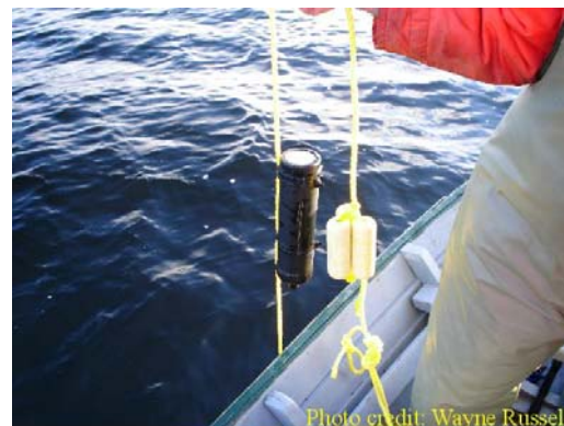
Figure 2. Autonomous receiver used for recording the movements of Gilbert Bay cod.
